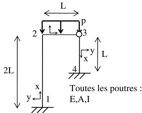
$$\text{barre 1-2 } \Omega_1 = 0, \Omega_2 \quad \text{barre 2-3 } \Omega_2, \Omega'_3 \quad \text{barre 3-4 } \Omega'_3, \Omega_4 = 0$$
