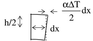
$$R = \frac{h}{\alpha \Delta T} \quad (\text{Rappel : } \frac{1}{R} = \frac{d\omega}{dx} = \chi \text{ Courbure})$$
