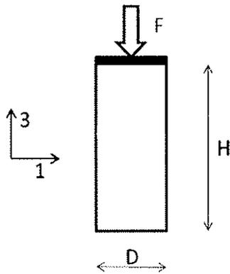
Figure 1 : essai de compression simple,  $H=100$  mm,  $D=50$  mm
