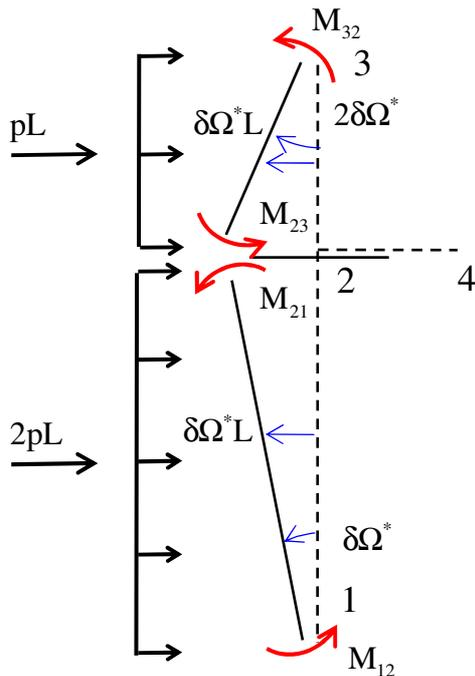
$$(M_{12} + M_{21})\delta\Omega^* - (M_{23} + M_{32})2\delta\Omega^* - pL\delta\Omega^*L - 2pL\delta\Omega^*L = 0$$
