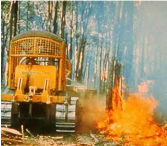
Figure 7- Bulldozers are used to clear breaks ahead of bushfires, even when a bushfire is active !
